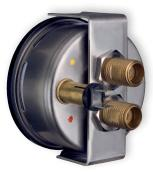
Including restrictor screw in each pressure inlet port, orifice Ø 0.8 mm (0.03"). Each process connection is marked with a coloured dot, matching the colour of the respective pointer.
